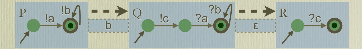
Network of finite automata communicating over *unbounded* FIFO channels.
